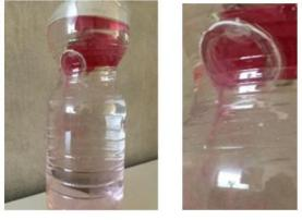
Figure 7: Introducing cold water at the top of a large container of hot water
