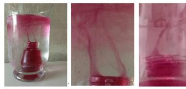
The less dense hotter water flows swiftly upwards forming eddies like plumes of smoke. The coloured water spreads outwards, forming a floating layer of warmer water at the surface (see Figure 4).
