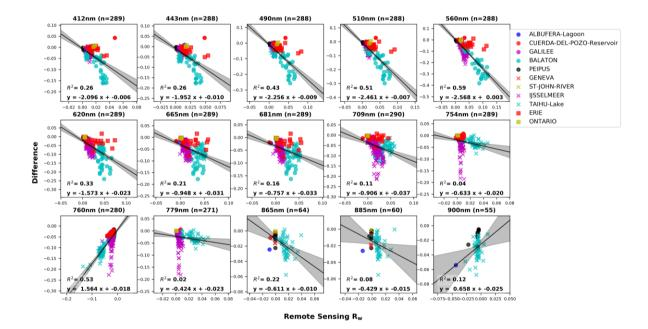
Figure 20 Linear correlation between Remote sensing Rw and the Difference between in situ and remote sensing Rw matchups (among which the wavebands of 865, 885 and 900 nm are not included in the Rw uncertainty products because of the sparse matchups).
