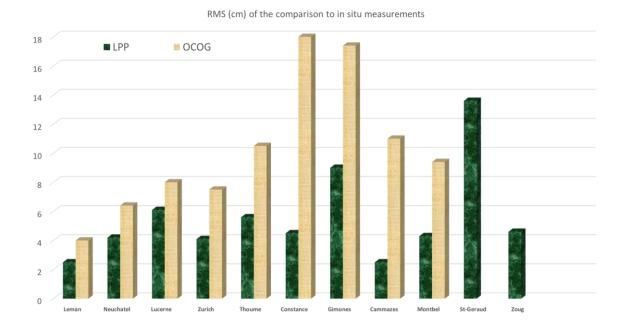
Figure 2: summary of RMS differences between in situ measurements and WSH calculated using LPP and OCOG retracker, for lakes in Occitanie and Swizterland.
