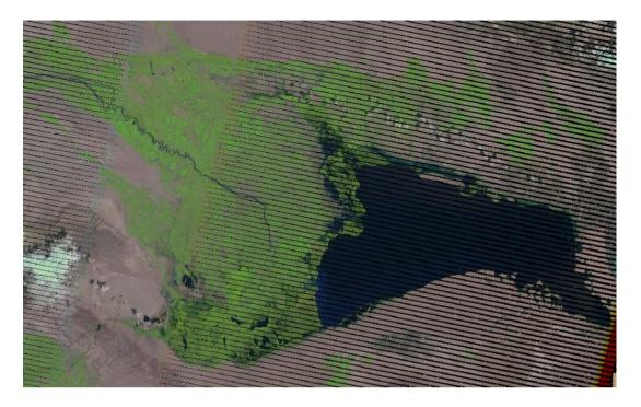
Figure 9: detectors errors on landsat 7 sensors acquired on the 2003-08-09 over Bosten lake
