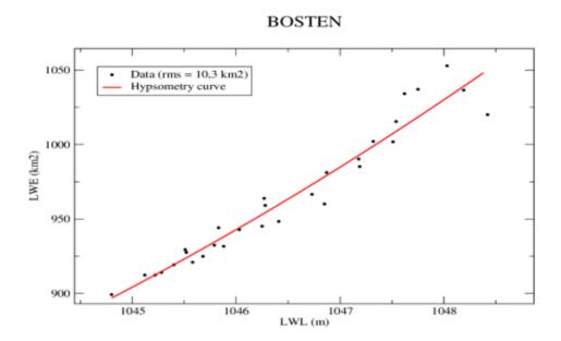
Figure 12: the hypsometry accuracy on Lake Bosten. Red curve represent the theorical hypsometry determined by least square adjustment of a second order polynomial on the datasets (LWL/LWE). With a 10.3 km² of RMSE this represents approximately 1% of total area of the lake.
