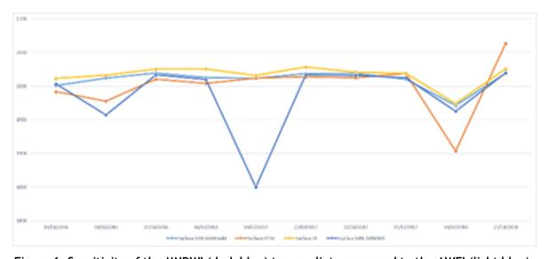
Figure 6. Sensitivity of the MNDWI (dark blue) to sun glint, compared to the AWEI (light blue), yielding a reduced water surface area in case of MNDWI for the sun glint affected scene on 14 July 2017 (low point in time series) shown in Figure 3
