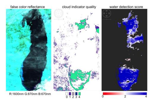
Figure 14 (Left) False colour composite image of reflectance at 1600 nm (R), 870 nm (G) and 670 nm (B). (Middle) the co-incident MERIS cloud indicator. (Right) The water detection score: QL 5 retrievals are made where this score reaches 4 or more. All panels for lake Michigan in USA on the 15-Feb-2011.
