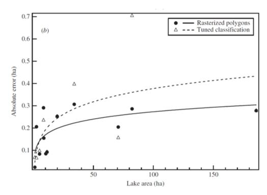
Figure 11: Scatter plots of absolute error in estimated lake area as a function of 'actual' lake area (based on DGPS shoreline measurements). Lines represent power-law fits to the respective data points (from Lyons et al. 2013)
