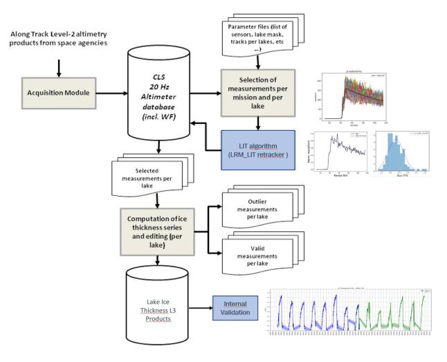
Figure 11. LIT processing system summary diagram
