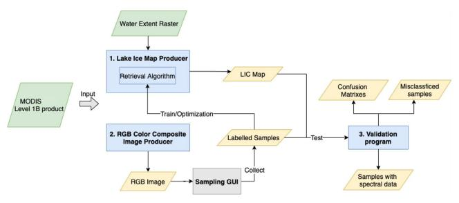
Figure 10. Overview of the LIC mapping system
