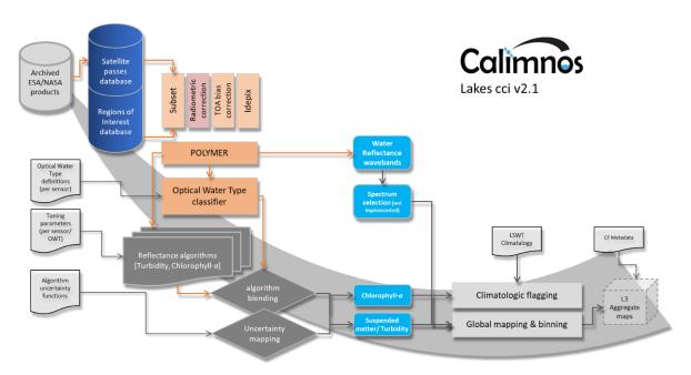
Figure 7: Schematic overview of the Calimnos processing chain for LWLR, Chlorophyll-*a* and turbidity or suspended matter.
