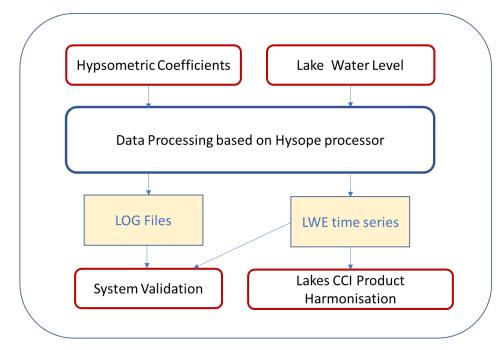
Figure 5. Overview of the elements and interfaces of the CCI Lakes LWE Processing Framework
