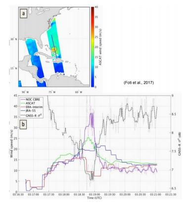
Ocean roughness and wind speed measurements 2-3 m/s RMSE (with hurricane penetration)
