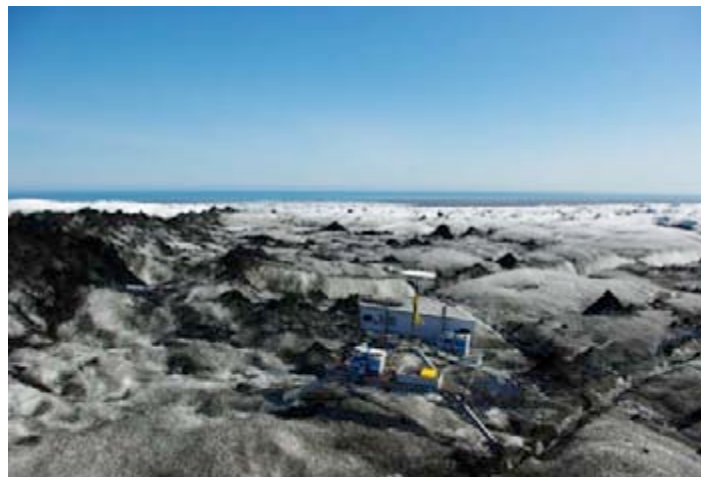
Figure 5.2: GPS Station BMJ2 with auxiliary energy supply by solar panels and batteries at Breidamerkurjökull facing southwards to the Atlantic Ocean (courtesy Eyjólfur Magnússon, Institute of Earth Sciences, University of Iceland).
