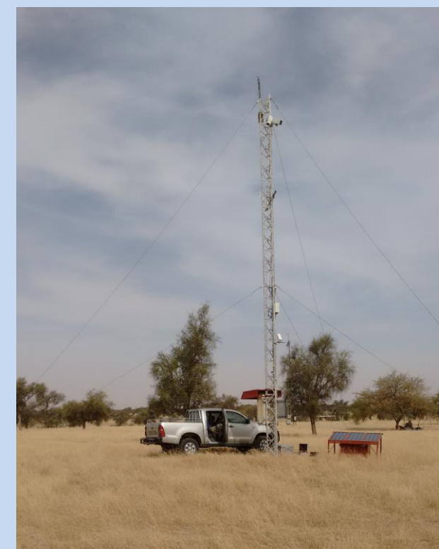
Fig. 3: Setup of Heitronics radiometers at Dahra, which will be re-installed by LAW. Photo from KIT.
