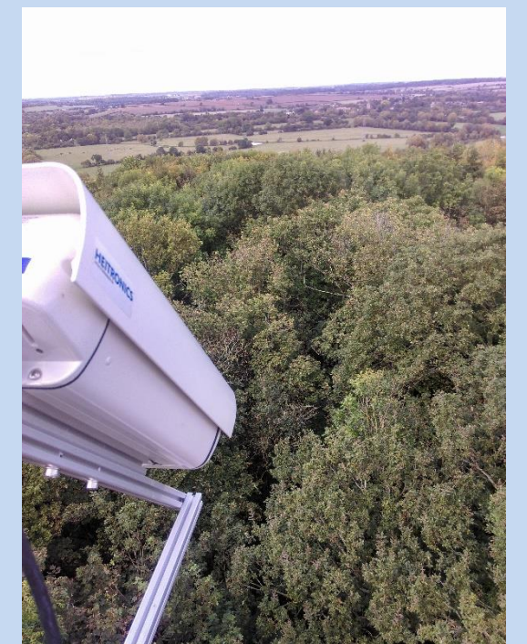
Fig. 4: Heitronics radiometer similar to those acquired for LAW deployed at Wytham Woods, Oxford. Photo from Emma Dodd.
